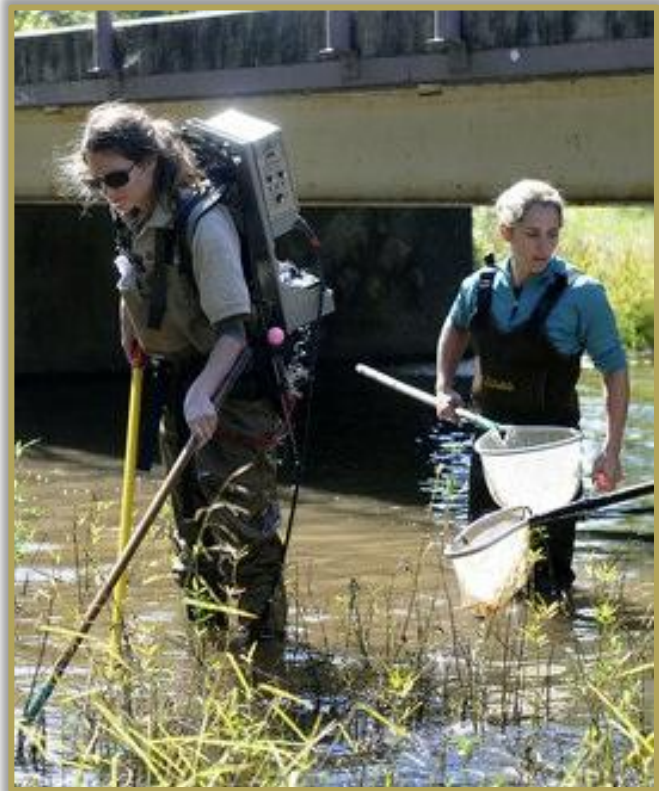
Figure 3.2.a. Fish sampling with backpack electrofishing equipment.
